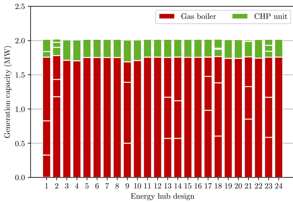
Figure 7: Installed gas boiler (nominal heating capacity) and CHP unit capacity (nominal electric power) for all 24 energy hub designs.
